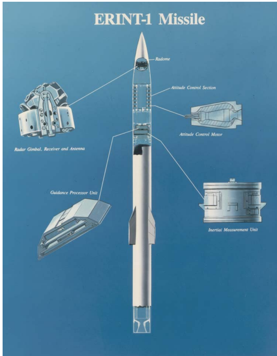
Fig. 5-9. The Extended Range Interceptor incorporated several technological advances creating a smaller, more effective interceptor.
